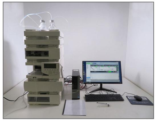
High-performance liquid chromatography (HPLC) is a technique used to separate molecules based on size and surface charge, among other properties. The incorporation of ultra-violet (UV) spectroscopy with HPLC allows the concentration of molecules to be determined following separation.
